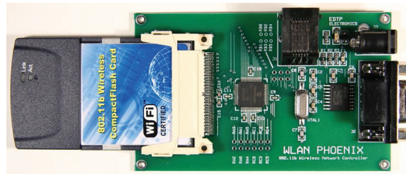
Figure 3. Airdrop-P system is a Microchip PIC18F6722 microcontroller based board with an 802.11b controller card
